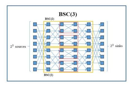
Figure 4: BSC(3), the 3<sup>rd</sup> Butterfly Superconcentrator.
