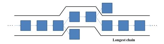
Figure 2: A schematic of the longest-chain protocol.
